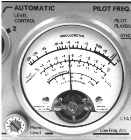
A reading of 0 dB on the Nagra would be nearly +10 VU on other recorders, which is a very hot signal!
