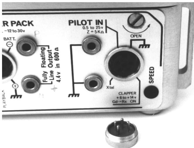
During normal resolve, the output of the crystal becomes the external sync reference.
