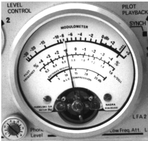
Think of it this way: the VU meter tells us **how far it is to the warning signs** and safety fence near the ravine, but the modulometer tells us **how far we are from the edge** itself!
